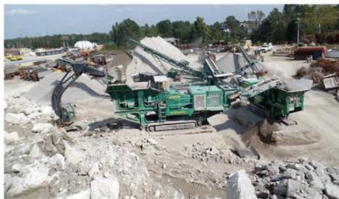
Fig. 1. Off-site concrete pavement recycling operation.
